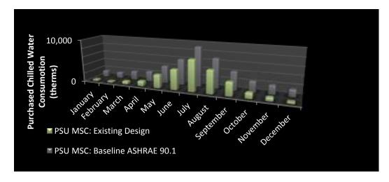
Figure 8: Comparison of Baseline and Existing Design Monthly Purchased Chilled Water Consumption
