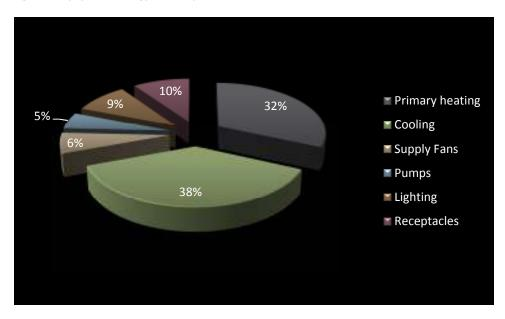
Figure 4: Equipment Energy Consumption: Existing Design
