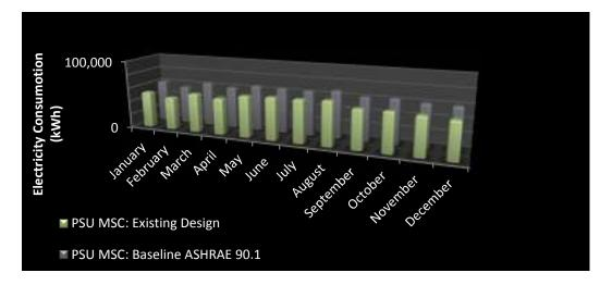
Figure 6: Comparison of Baseline and Existing Design Monthly Electricity Consumption
